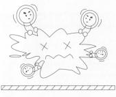
As ultrasonic waves pass through the solution in the tank, they cause rapidly alternating high and low pressures in the solution.
